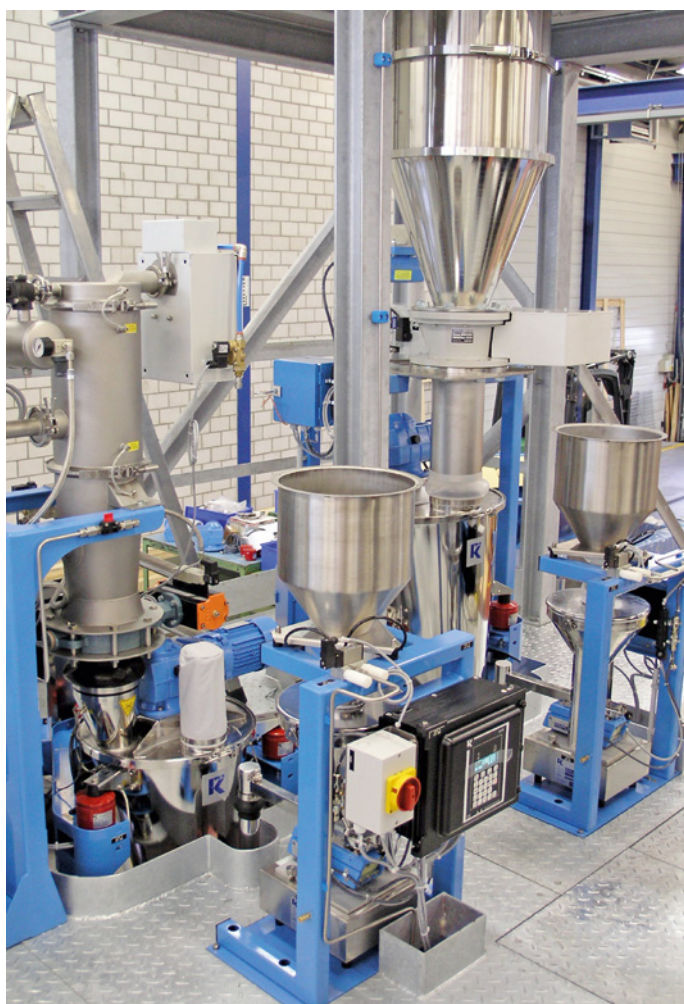
Coperion K-Tron feeding station with refill system
